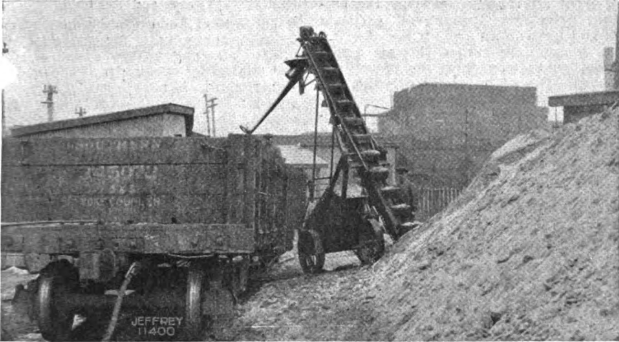
Type K Radial Loader used for handling material from storage pile to railroad cars. The swivel chute makes it convenient to distribute material over a greater area of the car without moving the loader.
